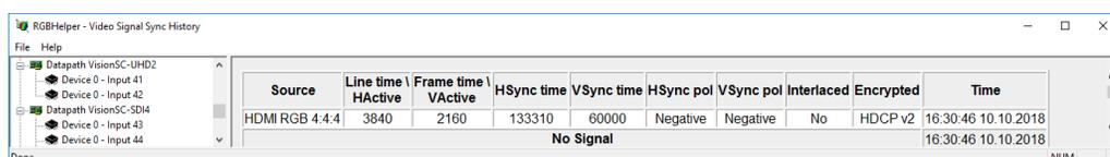
RGBHelper also allows the user to extract diagnostic information which may be useful to support staff should any problems arise with your XtremeDV-UH card. To create a diagnostic file open the **File** menu and select **Dump Diagnostics**. A dump file is then created and can be forwarded to EMS support staff.
