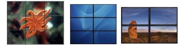
Bezel mask or screen border adjustment, this is quite an important function, normally the display will be 'staggered" from screen to screen due to the use of conventional LCD/Plasma displays, but with this function you can adjust the display to be seamless, e.g. mask-out the screen bezel enabling a visually seamless display.
